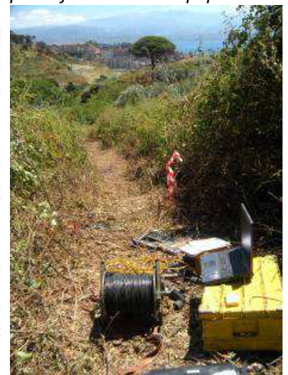
Map illustrating the trend of the higher part of the substratum obtained by the elaboration of seismic profiles. In the picture below a track of a seismic refraction profile and part of the utilized equipment
